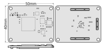
The XLM21 module series features Cologne Chip® GateMate® FPGAs packaged in a 4cm x 5cm module. Additionally, the modules contain on-board:
