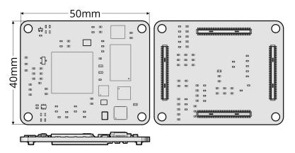
The XLM32 and XLM33 series features Efinix® Trion® FPGAs packaged in a 4cm x 5cm module. Additionally, the modules contain on-board:
