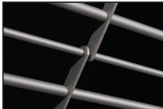
5/16" aluminum hoods rods spaced 1-3/4" O.C. with spacer tubes on every other rod and vertical links on 9" centers [optional perforated or polycarbonate panel available.]
