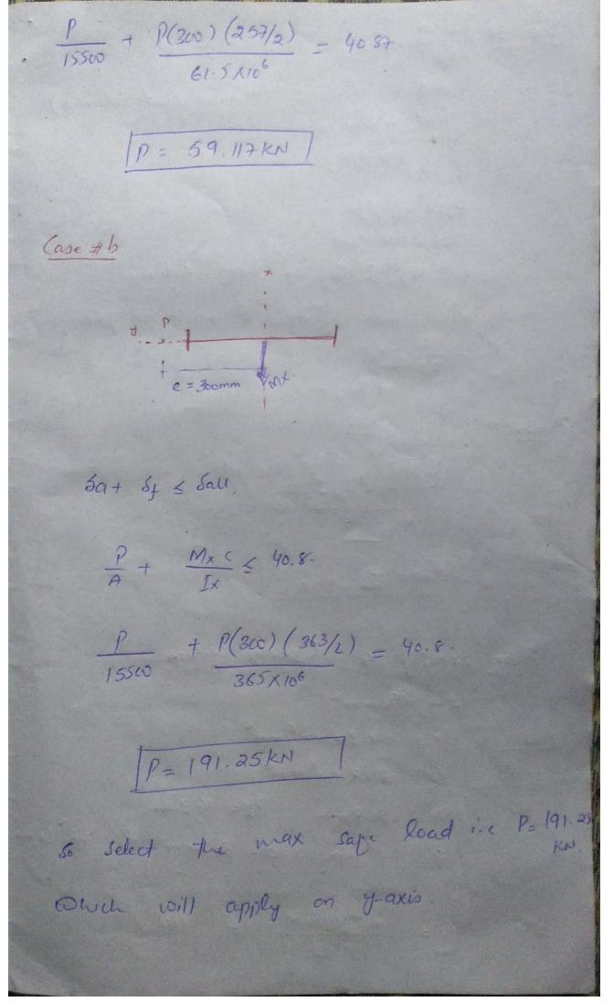
Pb#1139:- Given data. Section = CHOX45 (Hinged end Column). L = 2.2m P = 50KN. 5yp= 380Mpa. ST = 140 MPa E = 200 GP On which side & axis P must be placed? Rugx = ? Solution: From property of C310x45 section. A = 5690mm L IX = 67-3 m x 10 mm 4. It = 2.12 × 10 mm4 X= 17 mm. d= 305mm & bf= 80mn. to  $\frac{1}{\sqrt{y}} = \frac{2.2 \times 1000 \times 1}{19.3} = 114$
