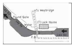
the Thames will pass through the pound, below the lock. The pound is used when the water level is low or for craft with a draught deeper than 0.54m (1' 9").
