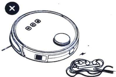
1. Power lines and other debris scattered on the ground may trip up product must be removed.
