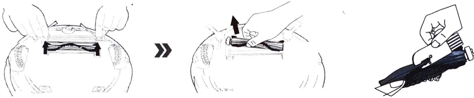
Set roller brush assembly: take out sucking assembly first, set the roller brush, cover the board and press it to lock.
