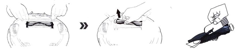
Set roller brush assembly: take out sucking assembly first, set the roller brush, cover the board and press it to lock.
