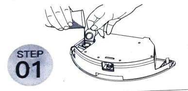
Sticking The Water Rag Close the water inlet cover and stick the water rag.
