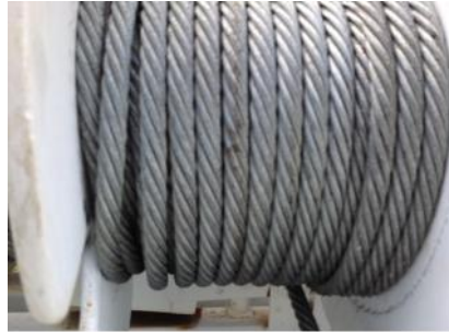
Example of correctly laid wire rope
