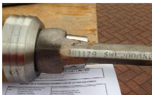
Lifting accessory showing unique identifier and safe working load (SWL)
