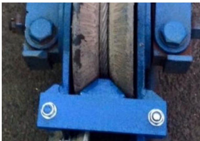
Example of V shaped wire rope retainer
