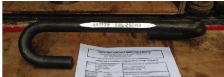
Lifting hook which should be used to tip the Shell
