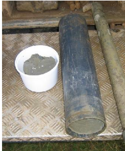
U100 shoe sample and U100 sample in a liner
