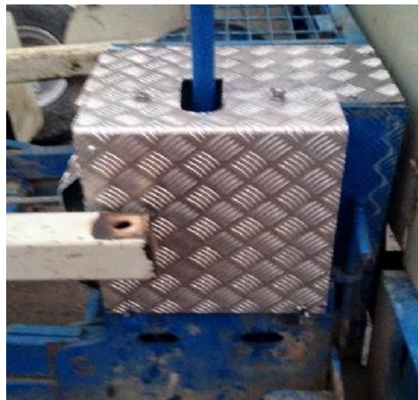
Example of clutch/brake guarding
