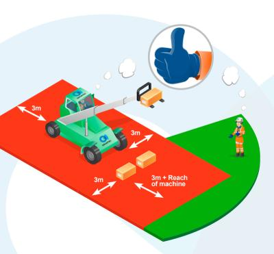
Red Zone: Keep out of this area at all times. No personnel to enter area unless the attachment is on the ground and the machine isolated.
