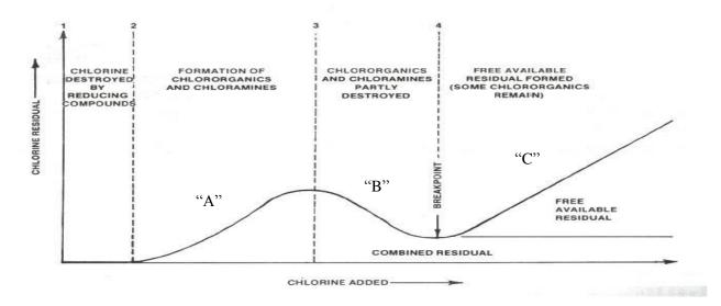
A common complaint received by many operators is that the water has a "chlorine odor." These odors are almost always caused by chloramines in the water rather than a free chlorine residual. Understanding the break point curve may help solve this problem.
