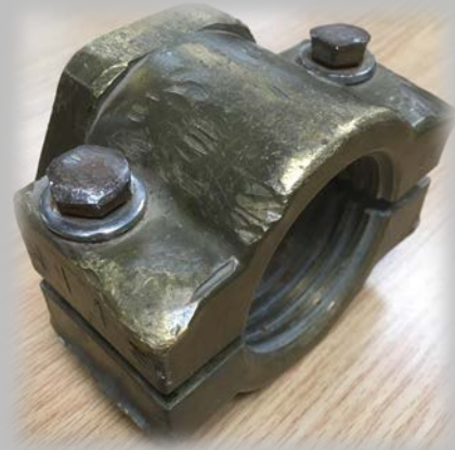
MI15 LIN CGA fitting after 18 month long term test
