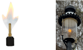
Flat-flame gas burners
