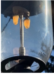
Double Mantle Inverted Welsbach Gas Burner
