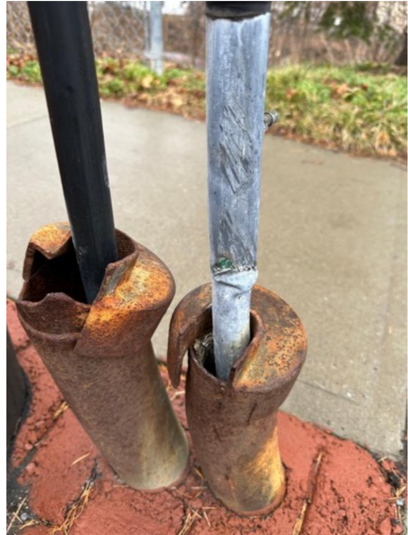
(L) Close up of damaged lead sheathed cable shown in (K). Wappingers Falls 3. January 2023, Wappingers Falls, New York.
