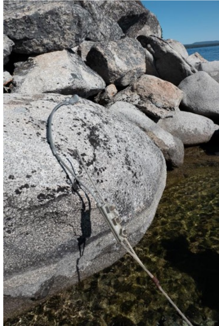
(F) Broken cable anchor on land near Rubicon. April/March 2022. Lake Tahoe, California.
