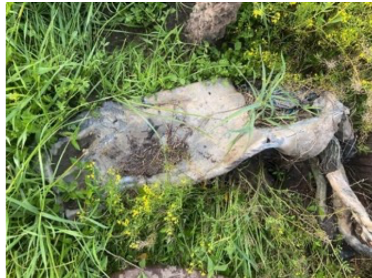
Figure 9 Photos. Louisiana continued. Damaged and abandoned leaded splice box and collection of five lead sheathed cables. MISS 12.3. June 2022, Donaldsonville, Louisiana.
