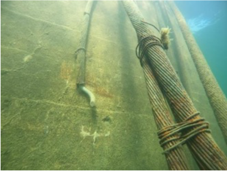
(E) Close up of small, cut, bare lead sheathed cable underwater. Site LP 4.1. August 2022, Lake Pend Oreille, ID.
