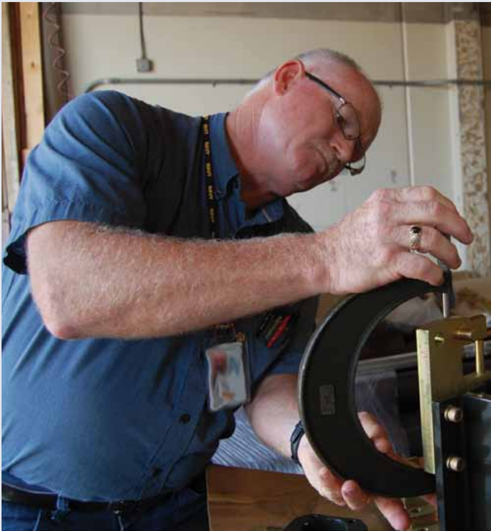
Don Carter, DCMA San Diego quality assurance specialist, inspects a machined part against the contract specifications to ensure it is within the specified tolerances. (Photos by Matthew Montgomery, DCMA Public Affairs)
