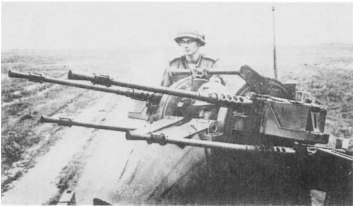
4 A quad 50 (four .50-caliber machine guns) mounted on a truck.
