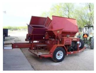
No matter which model of our worldclass CEB machines you decide to buy, in order to get the full capability out of your machine(s), you will need a good, efficient material mixing capability. Our Mega Mixer is the solution to the earthen construction industry's challenge of mixing a lot of earthen material fast, effectively, and for the long haul. This mixer has a large hopper for earth, a smaller hopper for
