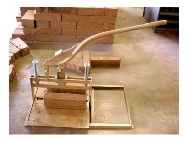
Our AECT block cutter makes straight cuts on un-stabilized CEBs (or stabilized CEBs that have not yet cured) in seconds. This device is simple to use and provides the user with a fast, repeatable, and effective way to cut blocks without the need for electricity or expensive blades.
