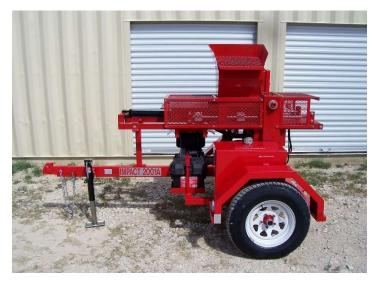
The Impact 2001A is the smallest, least expensive CEB machine that we make. This machine is automated and produces 300 CEBs per hour. It's fed by a smaller hopper that can be loaded using shovels, buckets, or a power conveyor. This machine is perfect for someone who only needs to build one to five houses. The Impact is lightweight and can be hauled behind any vehicle.
