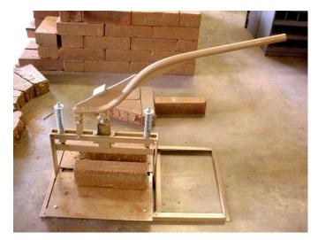
Our AECT block cutter makes straight cuts on un-stabilized CEBs (or stabilized CEBs that have not yet cured) in seconds. This device is simple to use and provides the user with a fast, repeatable, and effective way to cut blocks without the need for electricity or expensive blades.
