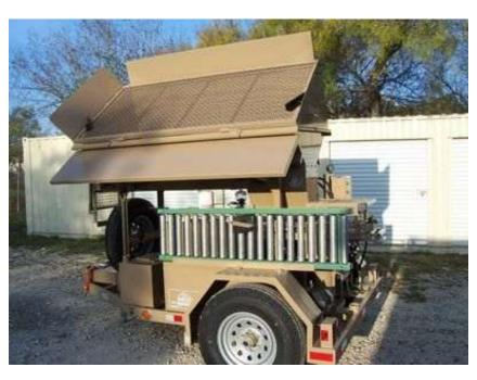
The 2500HD produces the same sized block as the Impact 2001A, but it produces 480 blocks per hour and has a one-yard hopper to facilitate loading with a tractor. If you like working with the 6" x 12" blocks, and you need to manufacture tens of thousands of blocks fast and without much effort, then the 2500HD is for you!
