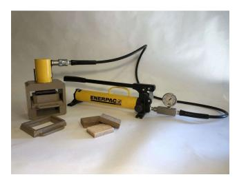
We manufacture the AECT Small Block Press at our factory in San Antonio, Texas. The Small Block Press tests earth samples over the same pressures and moisture ranges used by our full-size AECT CEB machines. This press operates over a pressure range of 1,000 to 6,000 PSI and produces a 2.5" x 3.5" x 1" earth block - a 1/4 scale size version of the typical 10" x 14" x 4" CEB produced by the AECT 3500 machine.
