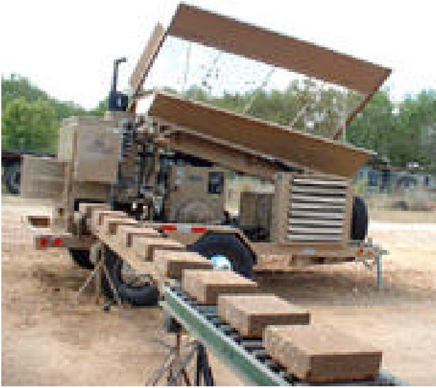
Figure 11. AECT 5000 Series Compressed Soil Block Machine
