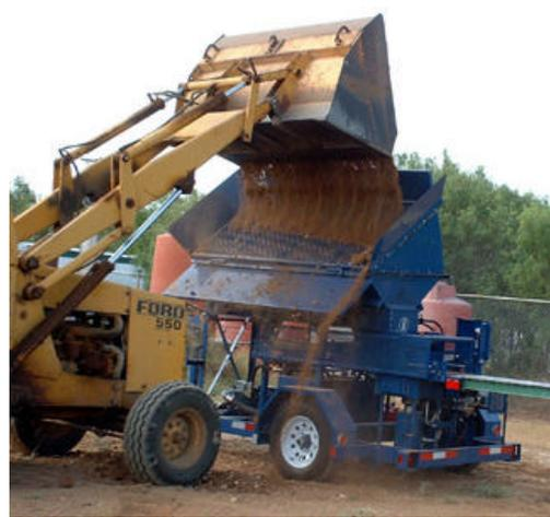
Figure 11. AECT 3000 Series Compressed Soil Block Machine
