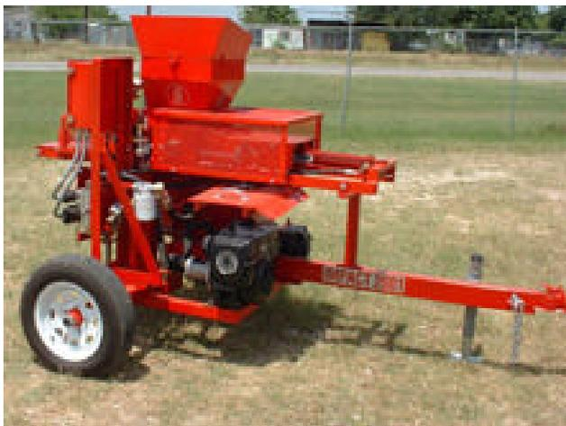
Figure 10. AECT Impact 2001 Compressed Soil Block Machine
