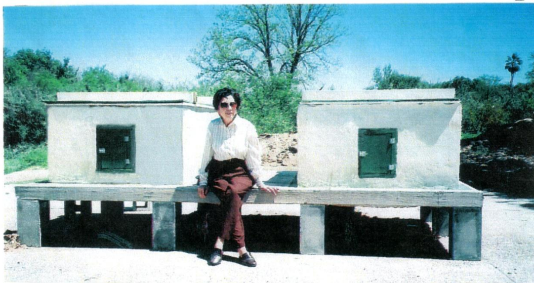
Figure 1. Experimental modules. Cinderblock left; adobe right. With ambient temperature of 98° F, temperatures inside the modules were 103° F for the cinderblock and 90° F for the adobe; a difference of 13°. The cinderblock was 5° F above ambient and the adobe 8° F below it. Recording of data was made 27 August 2004 at 4:30 p.m. Modules are located at the Casa de la Cultura in Del Rio, Texas.
