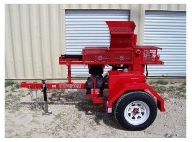
The Impact 2001A is the smallest, least expensive CEB machine that we make. This machine is automated and produces 300 CEBs per hour. It's fed by a smaller hopper that can be loaded using shovels, buckets, or a power conveyor. This machine is perfect for someone who is looking to build one to five houses. The Impact is lightweight and can be hauled behind any vehicle.
