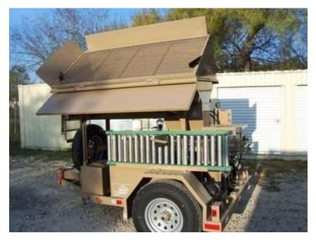
The 2500HD produces the same sized block as the Impact 2001A, but it produces 480 blocks per hour and has a one-yard hopper to facilitate loading with a tractor. If you like working with the 6" x 12" blocks, and you need to manufacture tens of thousands of blocks fast and without much effort, then the 2500HD is for you!
