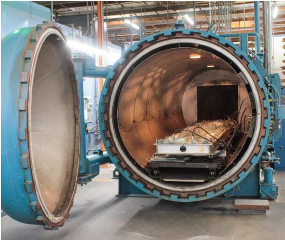
Figure 1 - Industrial autoclave during loading, with a composite component already vacuum-bagged on its tooling and prepared for the curing cycle.
