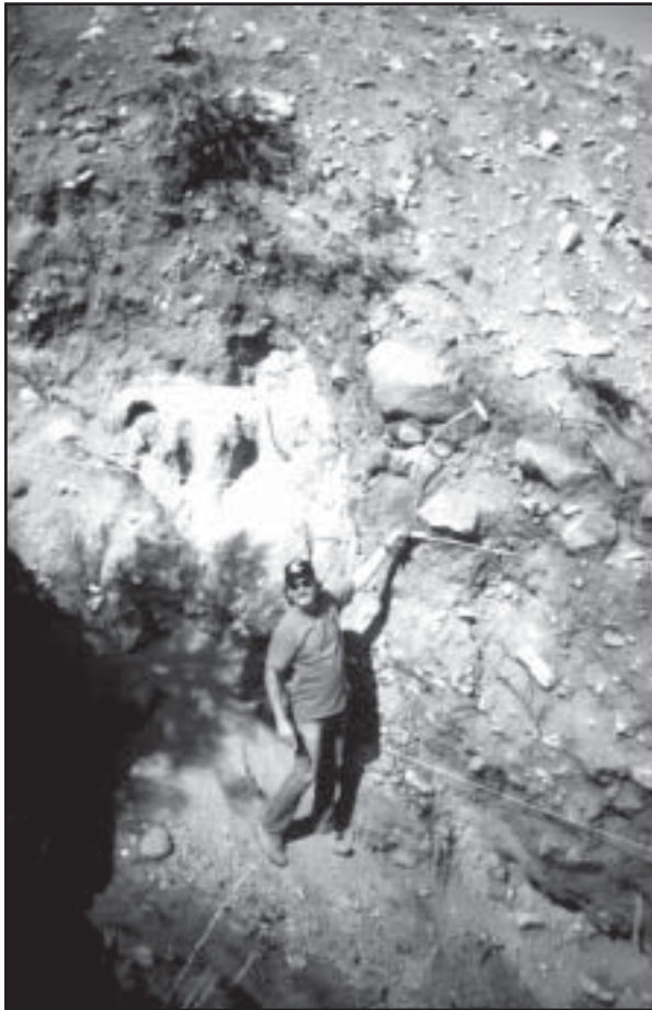
Figure 2. Backhoe trench along the Genoa fault near Walley's Hot Springs, south of the town of Genoa, Douglas County. The maximum displacement along the fault during its last event, about 550 to 650 years ago, was 18 feet (Ramelli and others, 1999). See www.nbmng.unr.edu/dox/sp27.pdf for Nevada Bureau of Mines and Geology Special Publication 27, a booklet on Living with Earthquakes in Nevada, for more information about earthquake hazards.
