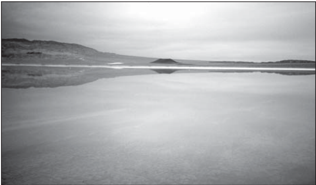
Figure 10. A Quaternary cinder cone at the north end of Clayton Valley, Esmeralda County, is reflected by the brine pool that is part of the lithium mining operation in the valley. Lithium-rich brines are pumped to the surface, where they are allowed to evaporate in the sun. The solution precipitates halite, NaCl, before being processed to remove lithium.
