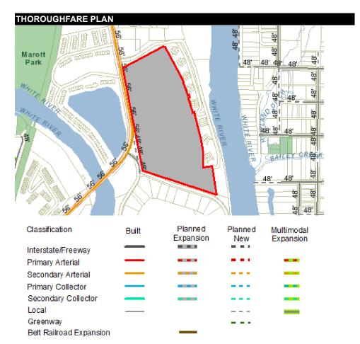
Numbers indicate proposed full right-of-way widths. If a "0" is listed, the proposed right-of-way is whatever the existing right-of-way is.
