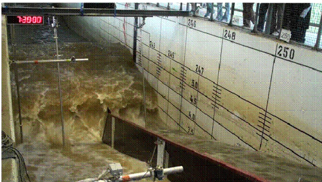
Figure 20. 74 th wave at t=450s (7:30min) just before impact on the revetment in GWK.
