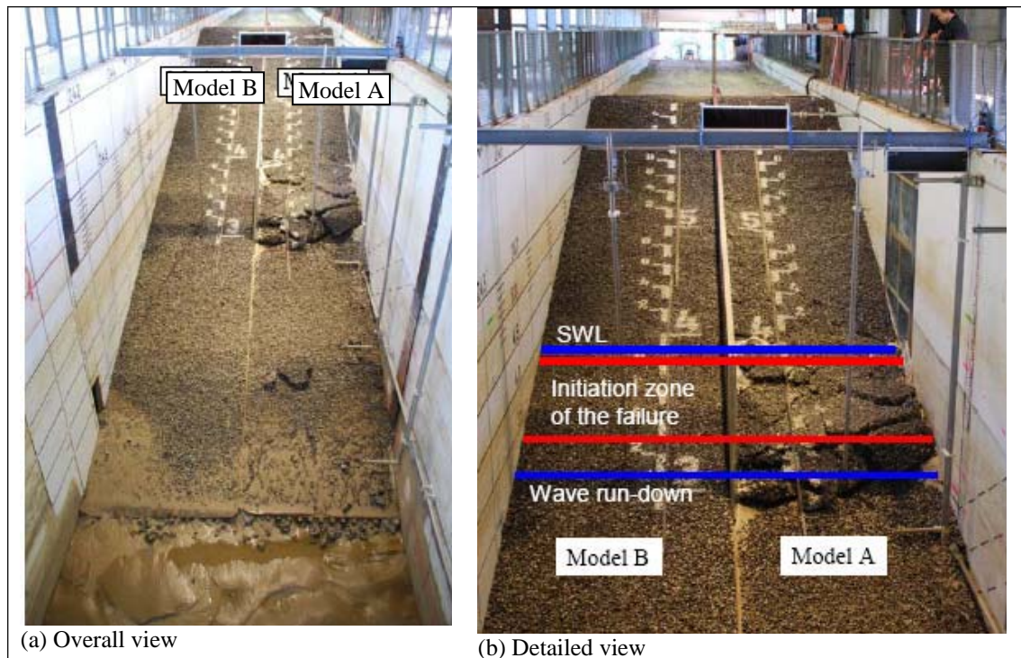
Figure 21. Extent of damage for revetment Model A after regular wave test 09051802.
