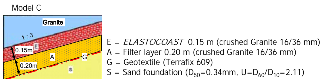
Figure 3. Model Alternative C (built after failure of Model Alternative A).
