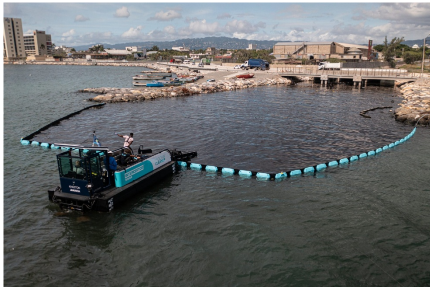
Image 3: Kingston Harbour, Jamaica - Interceptor Barrier with an Interceptor Tender (Courtesy of the Ocean Cleanup)
