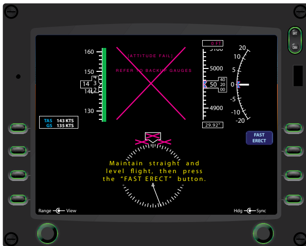
Figure 2-8. A PFD indicating a failed AHRS.
