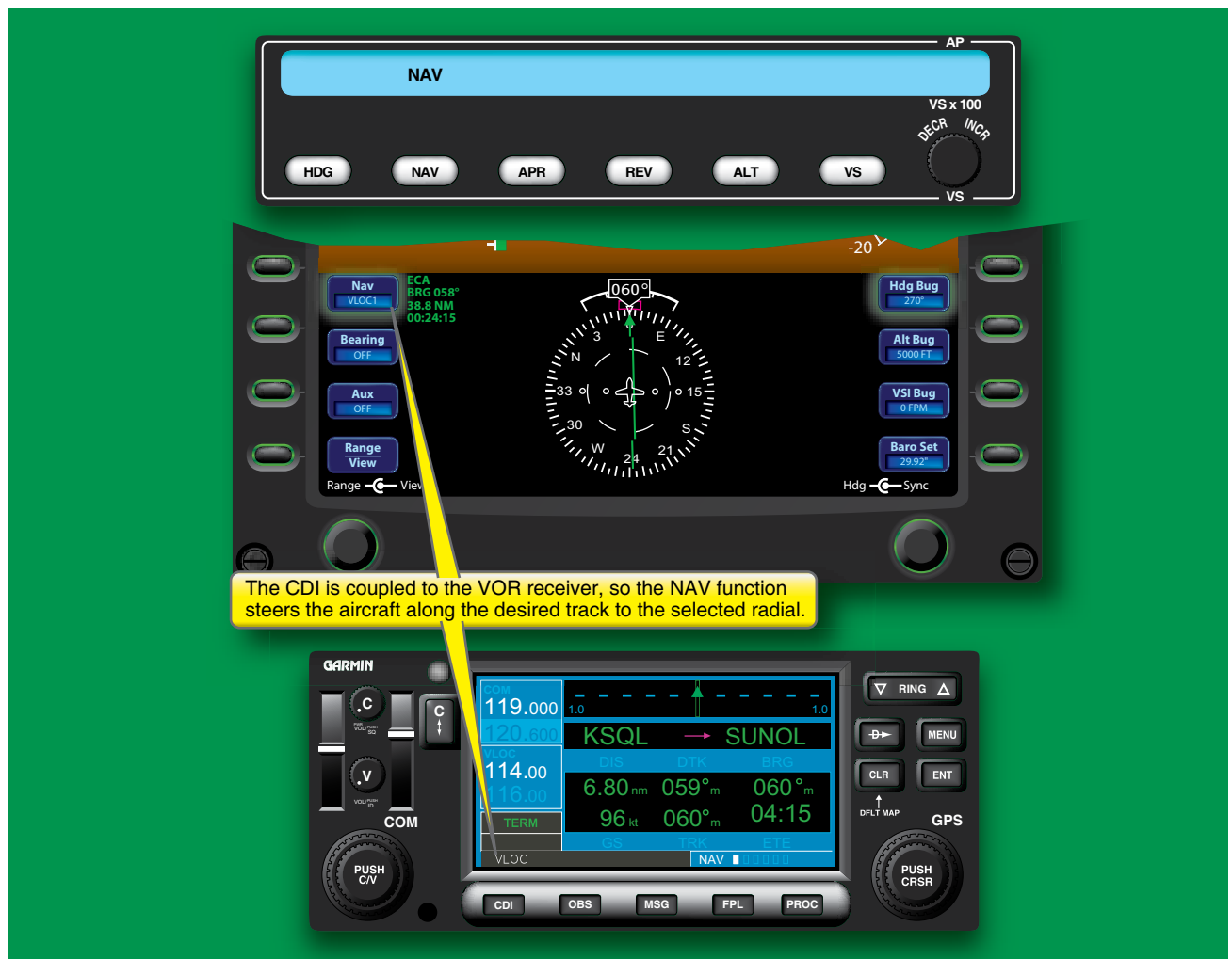
Figure 4-7. Using the navigation mode to follow a VOR radial.
