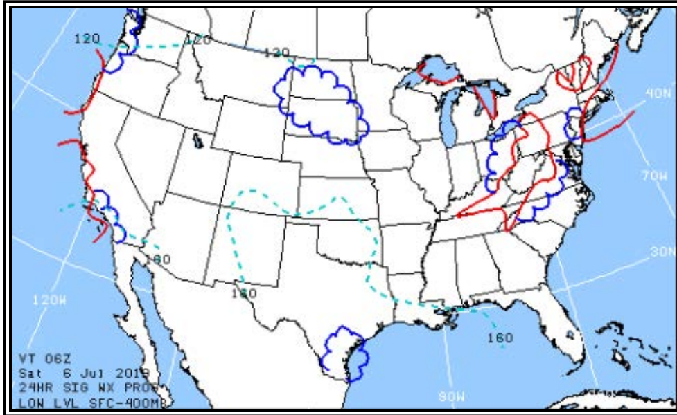
Figure 27-15. 12-Hour Low-Level SIGWX Chart—Example
