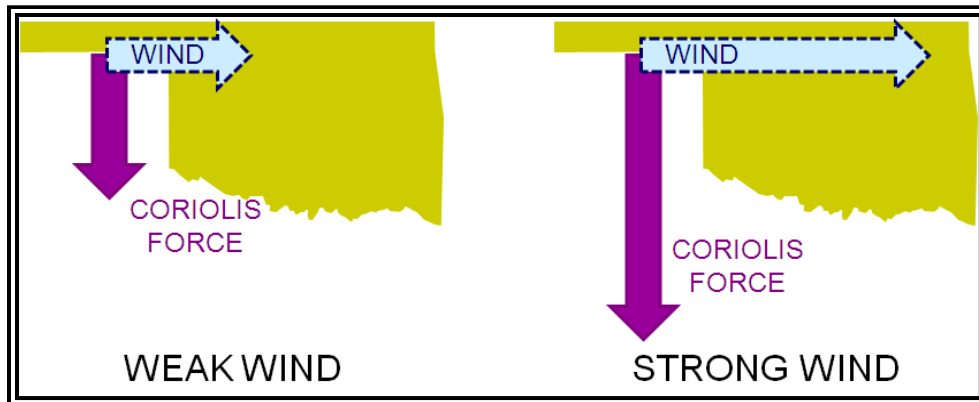
Figure 10-5. Coriolis Force Magnitude Variations with Wind Speed
