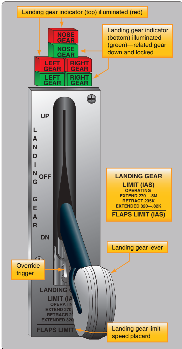
Figure 11-10. Typical landing gear switch with three light indicator.
