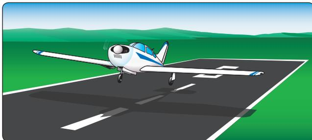
Figure 17-7. Landing with one main gear retracted.
