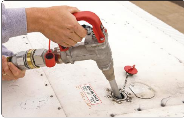
Figure 2-9. An AVGAS fuel filler nozzle is straight with a constant diameter.
