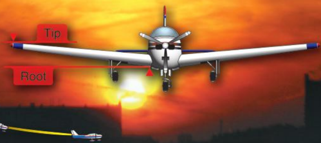
Wing Washout Wing root has greater angle of incidence than wing tip.
