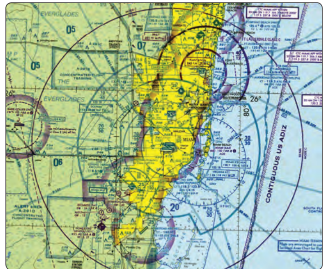
Figure 5-32. Temporary flight restriction (TFR).
