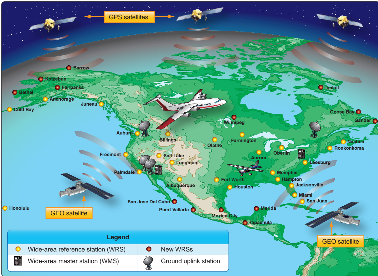
Figure 5-9. Wide Area Augmentation System (WAAS).
