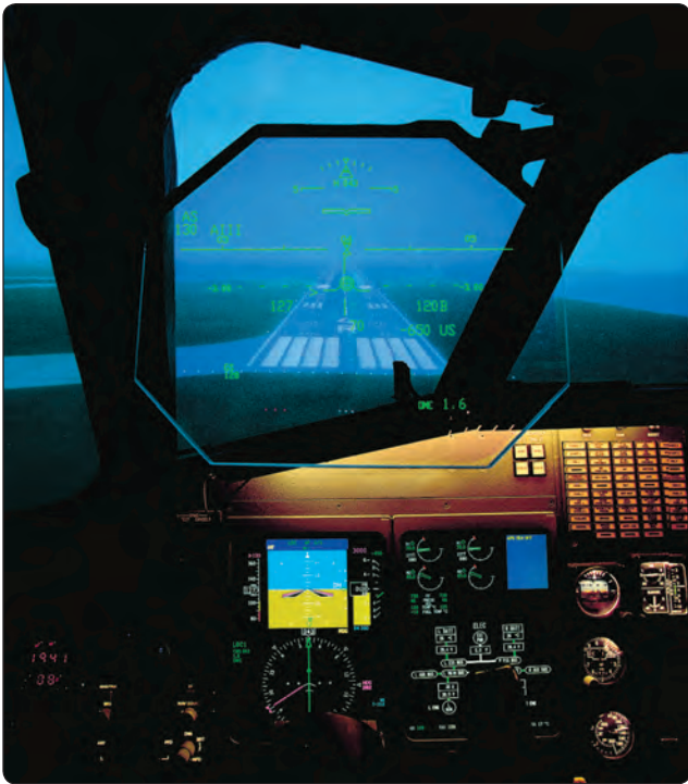
Figure 5-12. Head-up guidance system (HGS).
