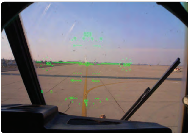
Figure 5-13. HGS using a holographic display.
