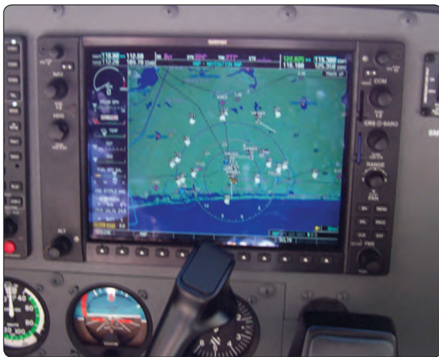
Figure 5-3. Automatic Dependent Surveillance-Broadcast (ADS-B) systems.
