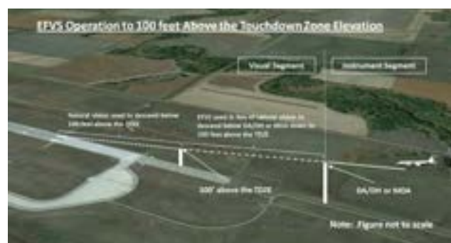
Figure 4-10C. EFVS Operations to 100 Feet Above the TDZE.
