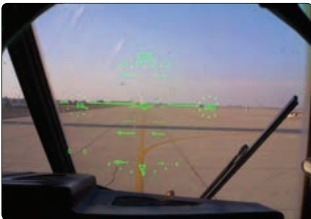
Figure 5-13. HGS using a holographic display.
