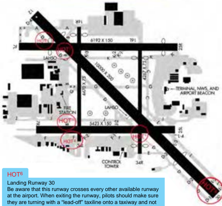
Figure 1-6. Example of runway hot spots located at Long Beach/Daugherty Field Airport (KLGB).
