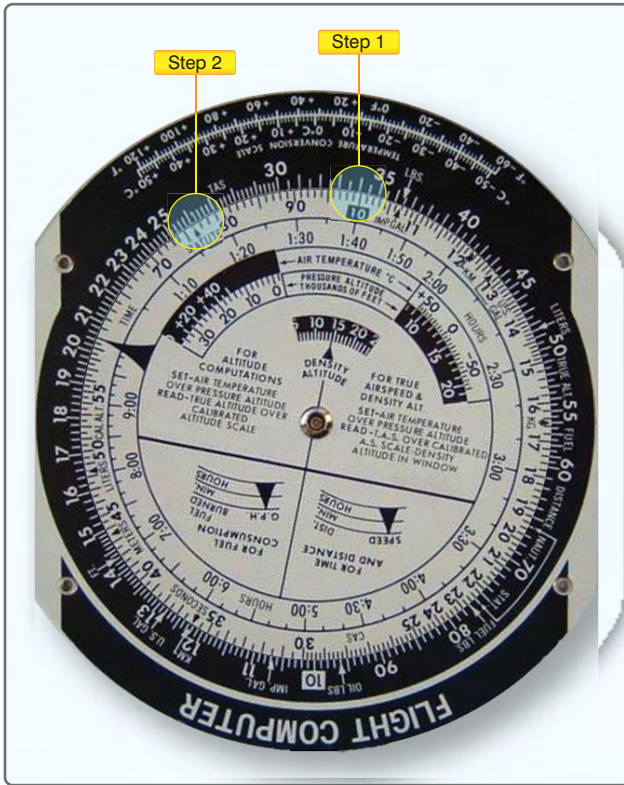
Figure 10-3. E6-B computer set up to multiply 340 by 78.
