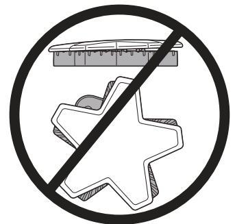
Incorrect burner cap
