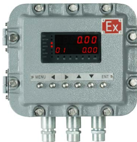
dCX-61-GM106-B68[U]EX [Explosion-proof/IP65/243×214×151mm]
