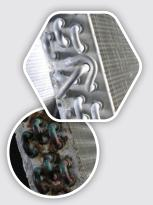
Traditional copper and galvanized steel coils are highly susceptible to corrosion.
