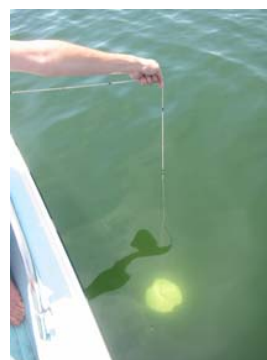
MEASUREMENT BEING TAKEN (Note the black measurement markings on the tape attached to the disk)
