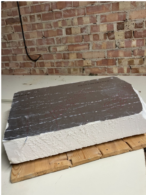
Poor quality and degraded EPS
