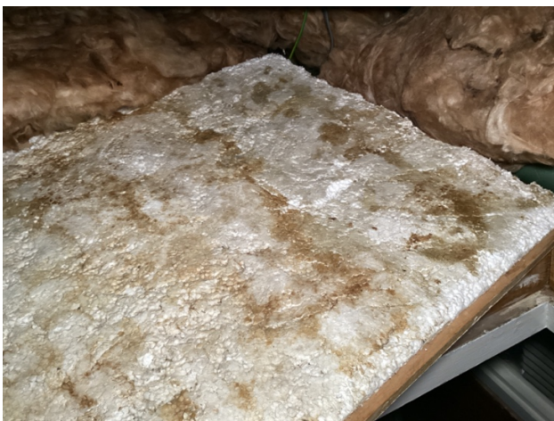
Poor quality and degraded EPS
