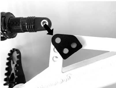
The position of the adapter plate in between shock and frame
