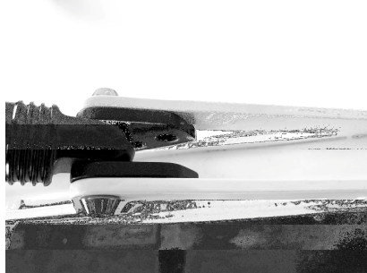
The adapter plates are mounted as a spacer only
