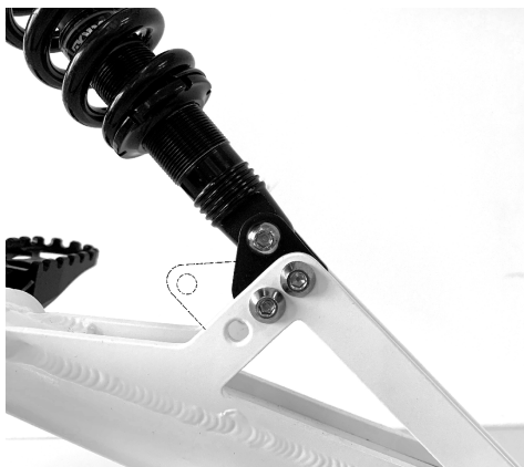
Adapter mounted and an alternative position
