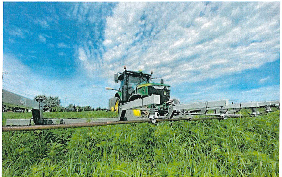
Herbicide resistance is becoming increasingly common— this NYFVI funded project is evaluating a non-chemical approach to weed management using an electrical discharge system.
