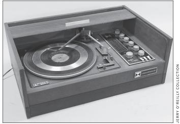
hink of the AD-27 as an uprated AD-17. The unit has a better turntable (BSR McDonald 500A or 510) and includes a receiver section (a modified AR-14); both also
