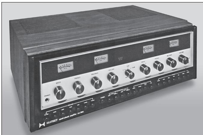
The AA-2010 replaced the short-lived AA-2004 in the January 1973 catalog. The distinction between the two is that the 2010 will decode all types of 4-channel program material without the need for any kind of external adapter. This was made possible with a more advanced decoder IC (an SN16800N instead of the of 87403 used in the AA-2004). Heath referred to the AA-2010 as a "universal 4-channel amplifier." Otherwise the AA-2010 and AA-2004 are identical.
