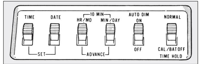
Figure 5. Bottom panel switches (D version).
