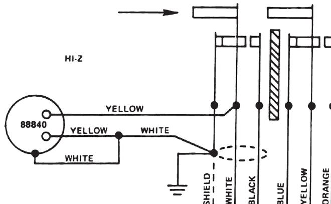
USE SHIELD AND WHITE WIRE FOR SHORTED OUTPUT IN OFF POSITION. USE SHIELD AND BLACK WIRE FOR OPEN OUTPUT IN OFF POSITION.
