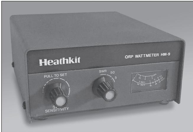
The HM-9 is another product designed for the QRP and VHF markets. It is a 50-watt power meter and SWR bridge that can be wired for one of three frequency ranges: 1.8-30 MHz, 50-54 MHz, or 144-148 MHz. The range is chosen during construction. It is built on a single PC
