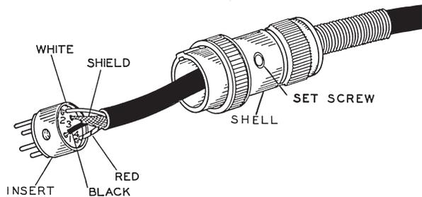
GH-12 microphone connections. Pins 1 and 3 are ground, 4 is PTT, pin 2 is audio.
