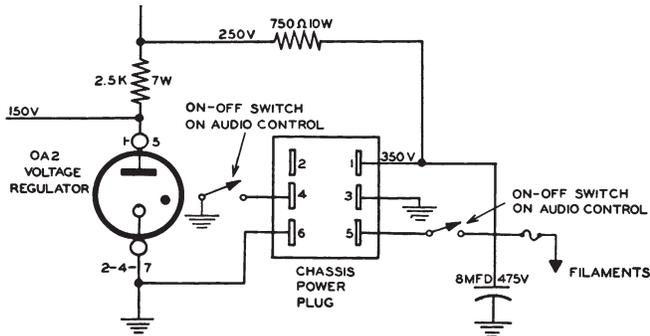
Figure 2. Detail of power connector and related circuit.
