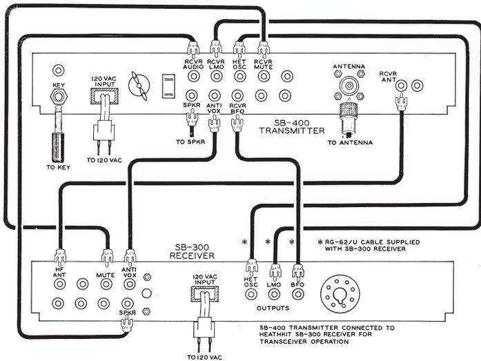
Figure 1B. Transceive configuration.
