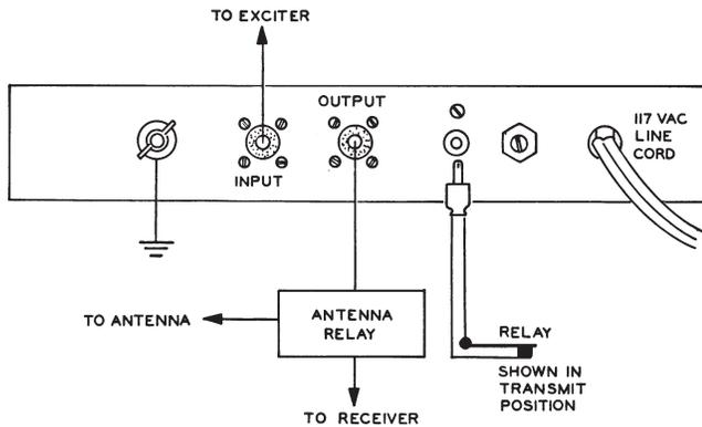
Figure 1. General arrangement of interconnections.
