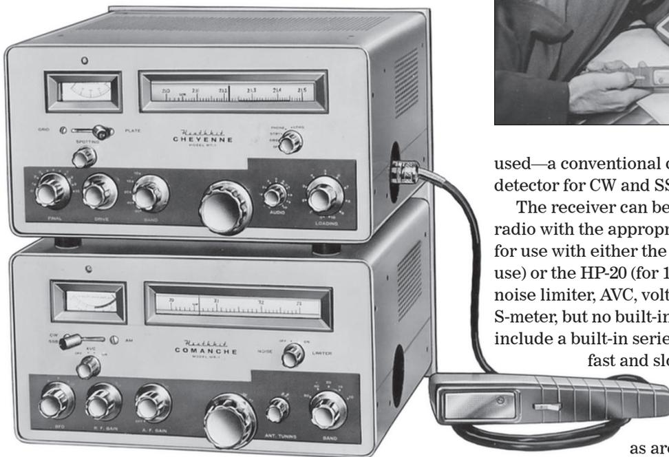
The MR-1 and MT-1 are matching rigs designed primarily for mobile operation, although fixed-station use is possible. A *QST* review marveled that the space occupied by both units was "a mere cubic foot."
