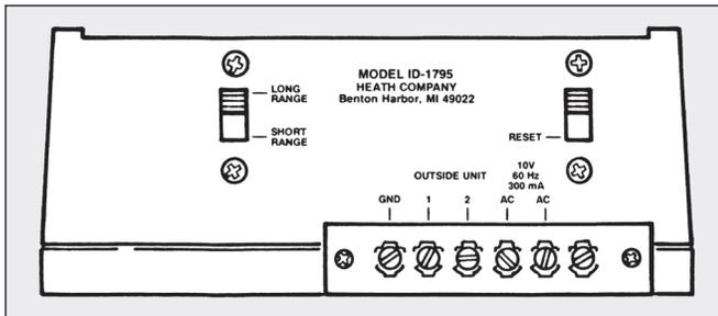
The ID-1795 was another huge success in Heath's line of weather instruments. The unit will measure rainfall in inches or centimeters, depending on the position of two jumper wires, which are easily changed. Refer to Figure 1. Note that changing from one unit of measure to the other will require recalibration of the collector bucket. A front panel LED indicates which units of measure are being displayed. LEDs are also used in the seven segment displays.
