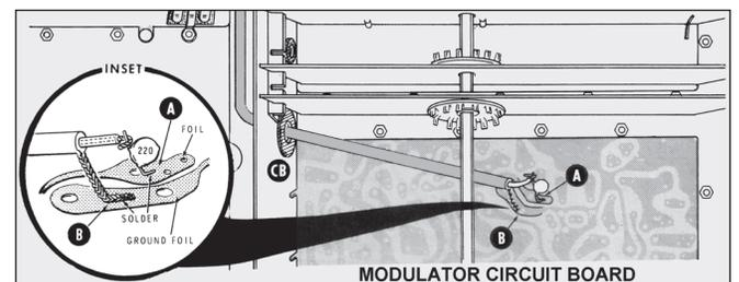
Figure 2. BFO Connection (SB and HW Series)
