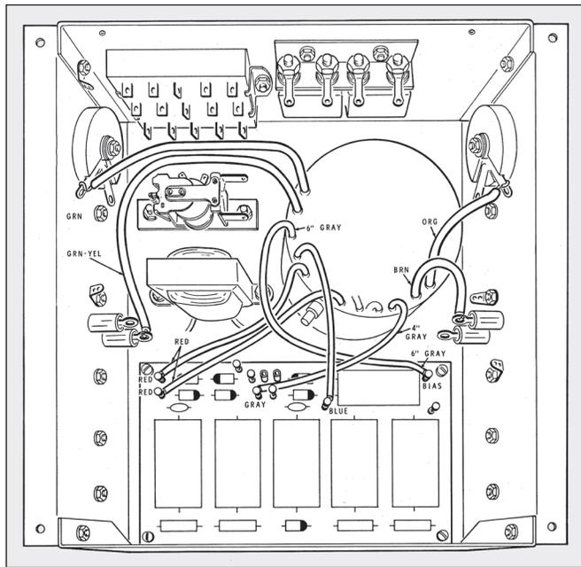
HP-13B. General arrangement of internal parts.
