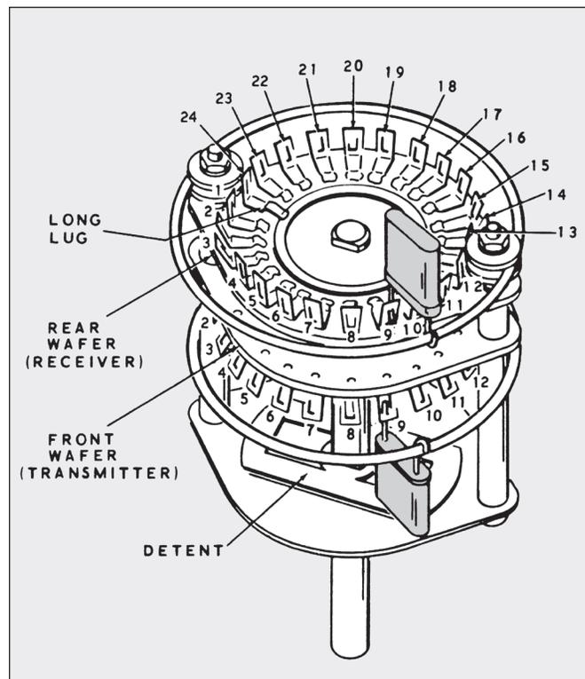
Figure 1. Detail of channel selector switch, with crystals installed for channel nine.
