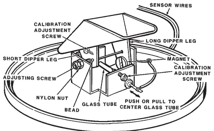
Figure 3. Detail of collection bucket tipping mechanism.
