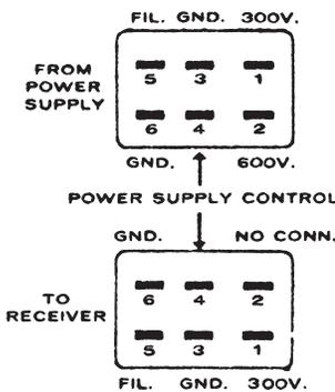
Figure 3. Rear panel power connections
