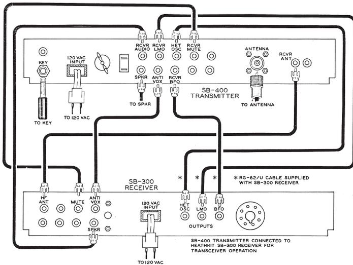
Figure 1B. Transceive configuration.
