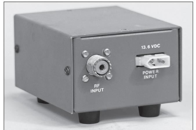
Released on the heels of the popular HA-202, this tiny Ramp was designed specifically to boost the signal from a handy-talkie. It provides about 8 watts of output with 1 to 3 watts of drive. The HA-201(A) is fully solid-state, no mechanical relays are used in switching. The amplifier will withstand infinite VSWR without failure but is not indestructible.
