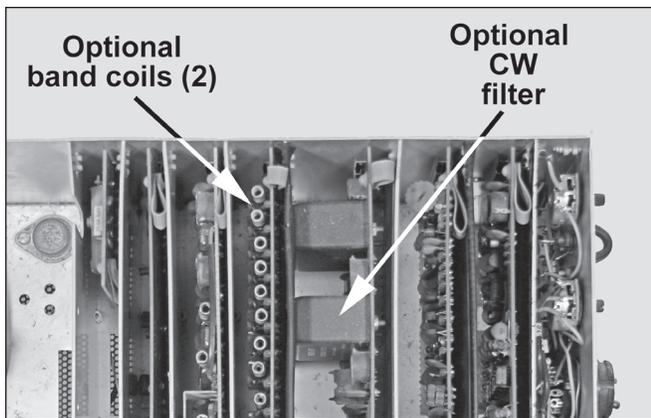
Figure 1. Location of optional band coils and CW filter.
