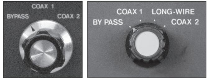
Figure 1. Detail of front panel showing added position on antenna selector switch of SA-2060A (right).
