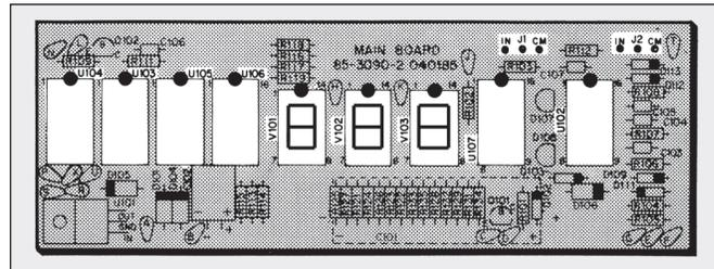
Figure 1. Location of jumpers (at upper right) required for inches or centimeters display.
