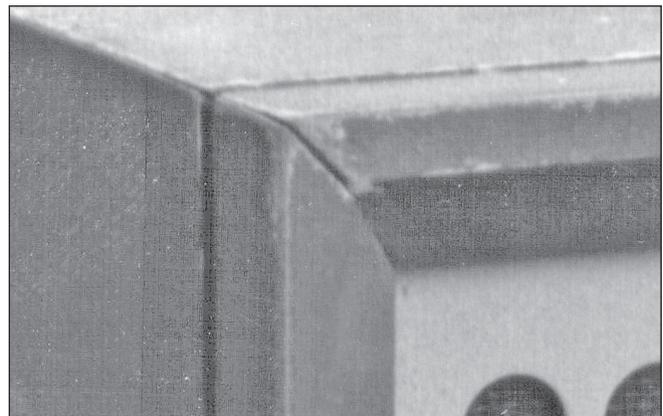
Figure 1. Note groove, which runs along the top and sides of the cabinet. Found only on the the first production run of the AK-5.
