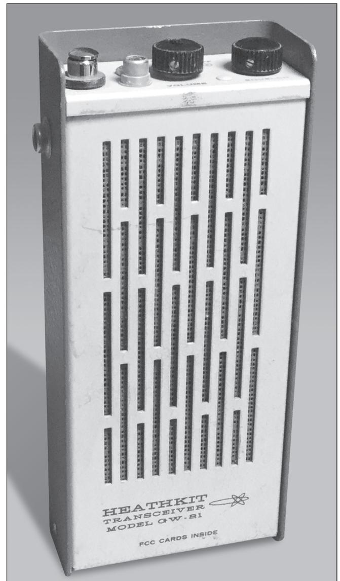
The GW-21 uses nine transistors and a super-heterodyne circuit, crystal controlled on one channel. Controls include on-off/volume, squelch and push-to-talk. Also includes jacks for an earphone and an external antenna. The crystals and all transistors mount in sockets.
