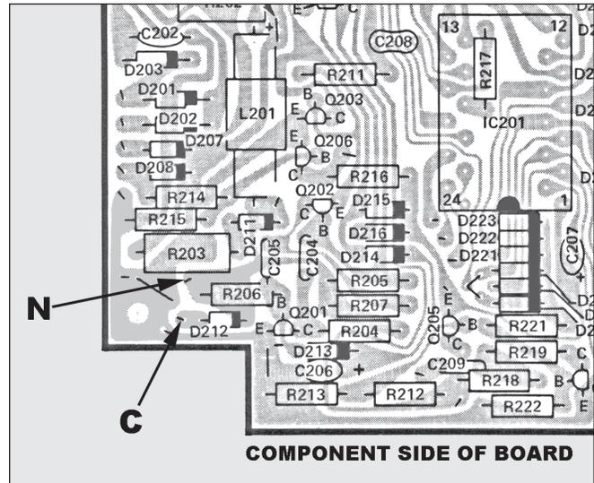
Figure 1. Battery type wiring options.
