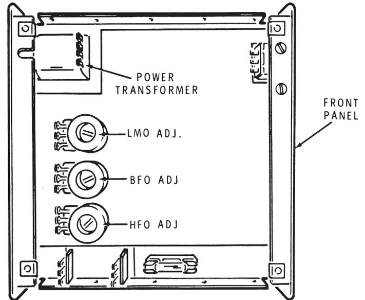
Figure 1. Location of level adjustments (on underside of chassis, left)
