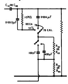
retained to provide a conducting path to the valve grid when the pickup heads are being interchanged.
