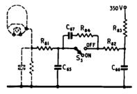
Fig. 18. Circuit of fading control.
