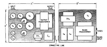
Fig. 4. Layout when using separate power pack.
