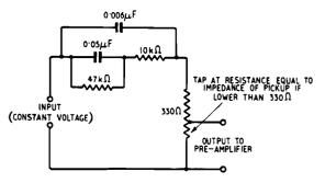
Fig. 32. Simulator for Decca 334 r.p.m. L.P. characteristic.
