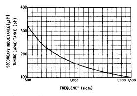
Fig. 21. Curve relating tuned circuit parameters and resonance frequency.
