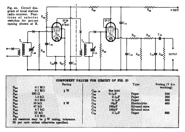
push-button or rotary switch. The use of variable inductors in this arrangement provides a simple method of achieving a uniform selectivity and sensitivity over the range, with the disadvantage that two coils or tuned circuits must be provided for each station to be received. In the unlikely event of serious thermal drift, correction is easily applied by the use of negative temperature coefficient capacitors.
