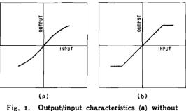
Fig. I. Output/input characteristics (a) without feedback (b) with negative feedback.
