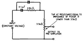
Fig. 31. Simulator for Decca and E.M.I. 78-r.p.m. recording characteristics.
