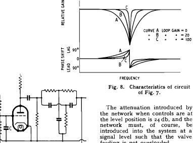
Fig. 7. Basic filter circuit.
