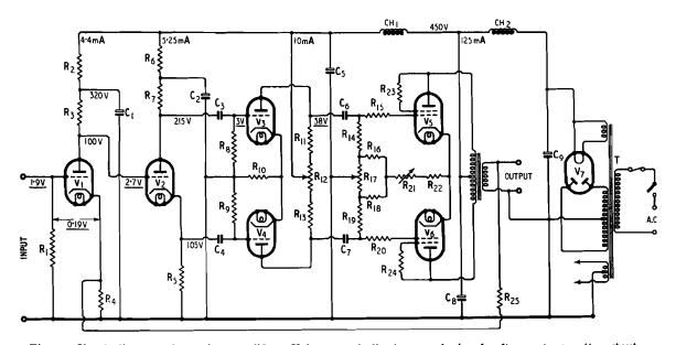
Fig. 5. Circuit diagram of complete amplifier. Voltages underlined are peak signal voltages at 15 watts output.
