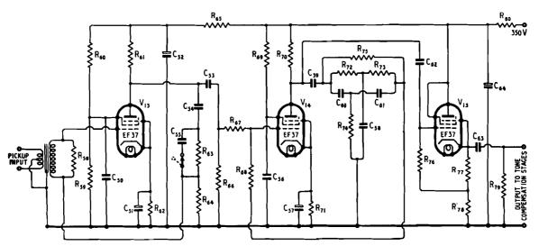
Fig. 15. Pre-amplifier with high-pass filter.
