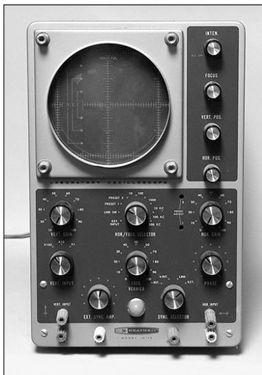
said “laboratory oscilloscope.” See IO-30 for details and specifications. Replaced by the IO-18 in 1968. Same tube complement as IO-30: (1) 6AB4, (1) 6AN8, (1) 6J6, (1) 6C4, (1) 12BH7, (3) 12AU7, (1) 6CA4, (1) 1V2, (1) 5UP1. Replaced in 1968 by the IO-18. Power: 80 watts. Size: 14 high x 8.75 high x 16 deep. Weight: 19 pounds.
