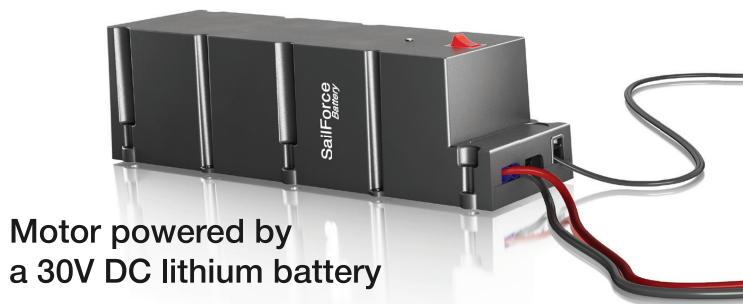
For optimal performance, the 12V DC (direct current) supplied by the service batteries is not sufficient. That's why the SailForce™ electric winch is powered by its own 30V DC lithium battery, with a capacity of 144Wh, which is more than enough to power one or two electric winches.
